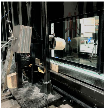
Impact Test on 4' x 6' Flood Window
