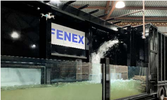
Filling Custom-Built Test Rig
