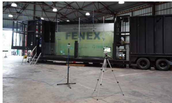
Load Test of 9' of water on 20' x 11' Flood Window
