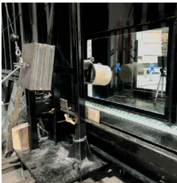
Impact Test on 4' x 6' Flood Window
